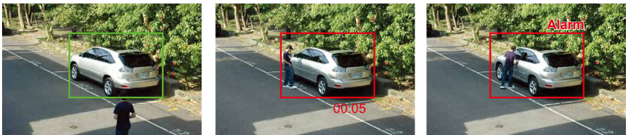
Figure 10.6 Alarm triggered by loitering detection
